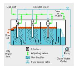
often experienced at the wellhead. Without chemical addition, flotation units should remove particles larger than 25 microns. With chemical addition to coagulate the oil and solids, particles less than 10 microns may be removed.
